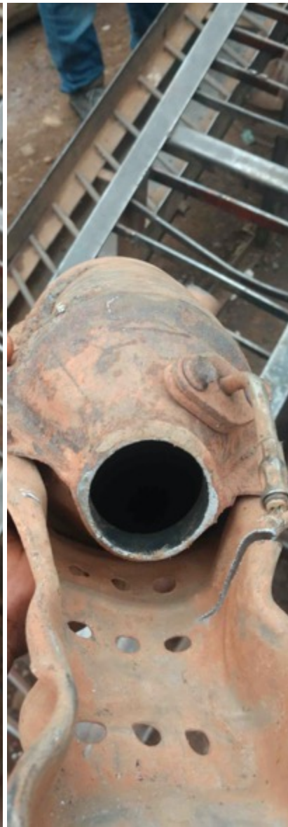
Modified or deleted catalytic converter by some African mechanics
