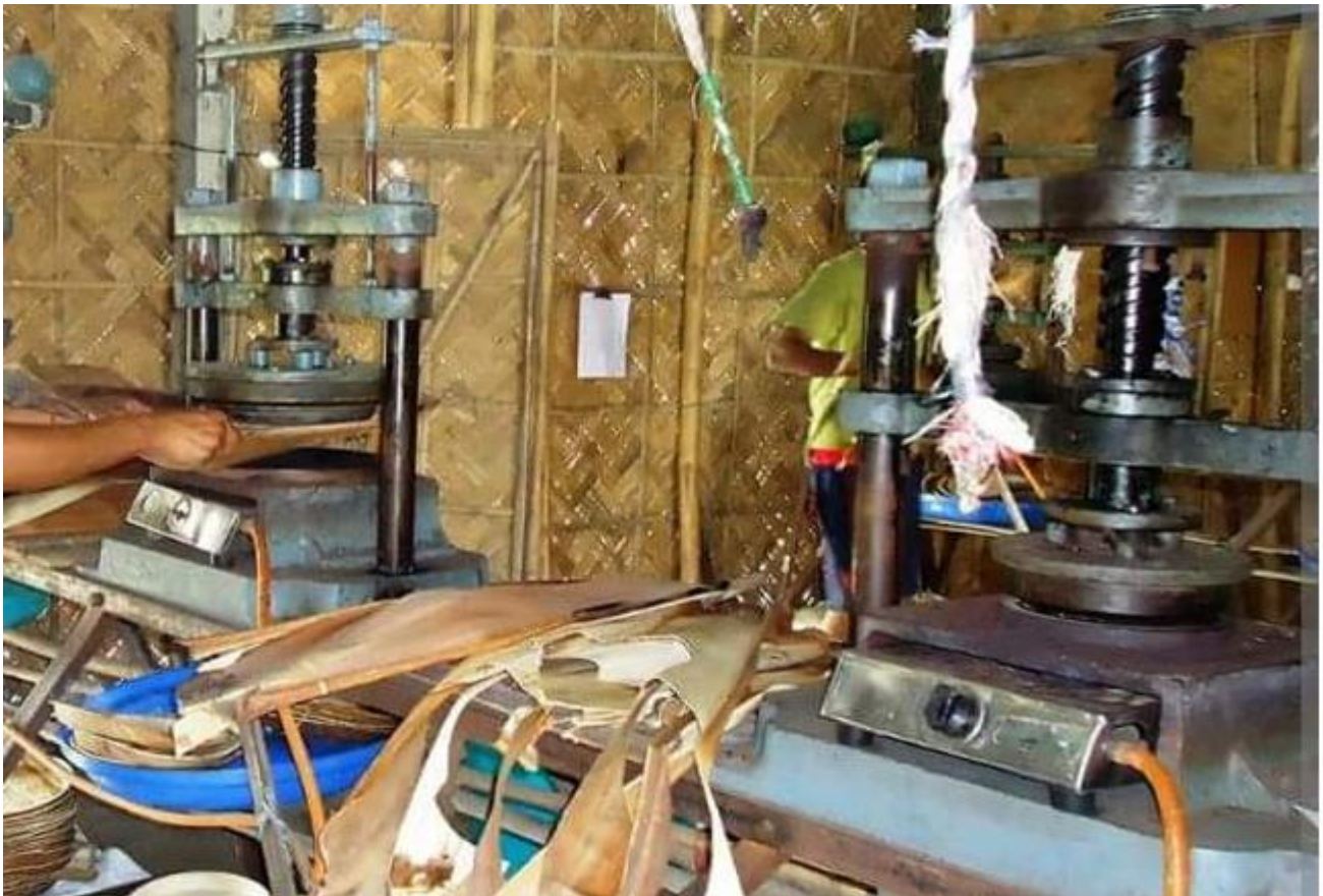
Picture – 4: Molding washed leaves with high pressure and temperature (We will upgrade)
