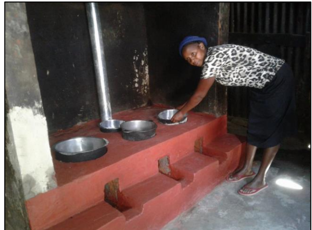
A woman fitting pots in her newly installed smokeless stove
